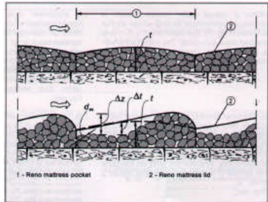
**Figure 2. Gabion mattress showing deformation of mattress pockets under high velocities (courtesy Maccaferri Gabions)**
