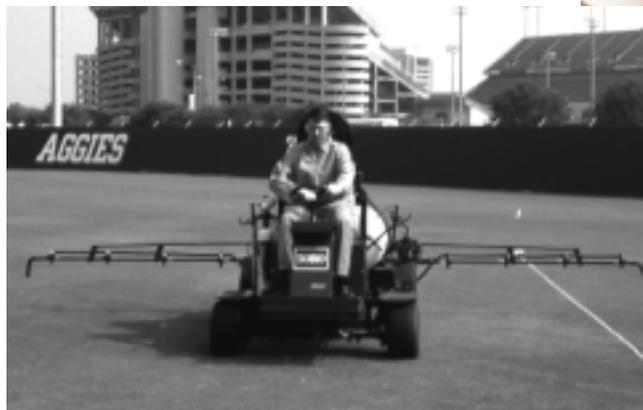
Drive the 200-foot distance with the tank half full, and at desired RPM and gear settings.
